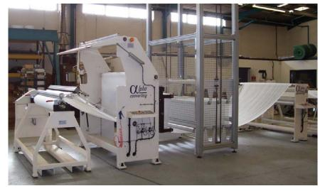
This ALPHAREEL mated with an existing process line. It features automatic closed loop tension control to minimise stretching or elongation of the web and is fitted with an accumulator to provide continuous line running at full speed during reel change over.
