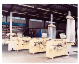
The ALPHASPOOL SPD with accumulators for continuous running. The accumulators allow a full spool to be replaced without stopping production.
