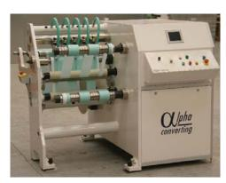
ALPHALAB TWIN – a narrow width slitter with individual dust extraction for each knife.
