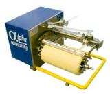
General purpose ALPHATRIM for winding edge trims at speeds up to 600 m/minute.
