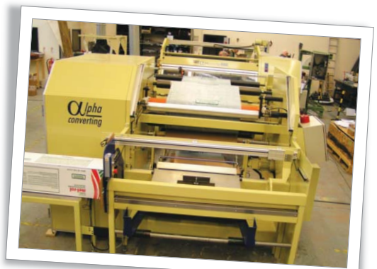
Finished rolls automatically loaded into a box on a single position ALPHAMATIC reduces operator handling
