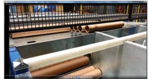
Automatic core loader accepts different core lengths for flexibility of slitting widths
