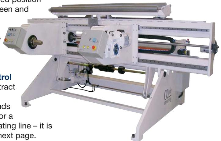
**The ALPHA REEL unwinding and rewinding system for wovens / nonwovens uses advanced technology and multi-tension zones for lightweight and extendible materials.**
