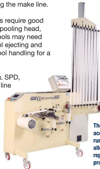
Alpha Converting supplies slitting and spooling equipment for a very wide range of products, with each machine engineered to optimise the efficiency and quality of the process. All its spoolers have an easy operator interface for selection of the spooling pattern, with computer control of the pattern for accurate and repeatable lay down of the tape or yarn.
