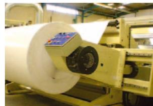
Pick up unwinds with tension control through precision disk brake or motor drive. Option for shafted unwind. Unwinds may be integral to slitter for space saving and reduced cost or separate for larger diameters and improved access.
