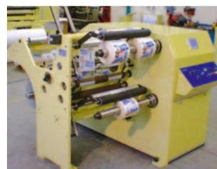
The ALPHATWIN is available with a cantilevered winding shaft for narrow webs.
